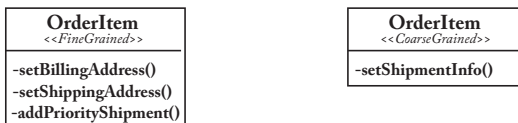
(a) Fine-grained version exposing different methods for setting each different needed information.
