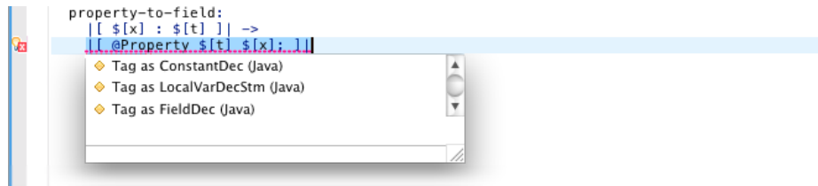
Fig. 1. Screenshot of a quick fix dropdown menu, listing three possible tags to disambiguate a Java quotation. The menu can be triggered by clicking on the error icon shown in the left margin, or by using a keyboard shortcut. Selecting a suggestion fixes the ambiguity.
